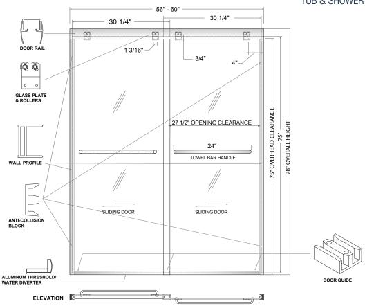
\*NOTE: These measurements are based on a standard 60"x78" enclosure. Heights and Widths are variable and can be ordered to fit specific project requirements.
