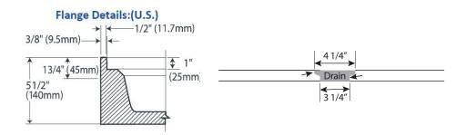
$\textbf{FEATURES} \ \ \textbf{Dimensional Tolerance} \ \pm \ \textbf{1}_{\textbf{8}^{\text{II}}}. \ \textbf{Dimensions needed for site preparation should be measured from the unit.} \ \textbf{American Bath Group assumes no responsibility for preparatory work.}$
