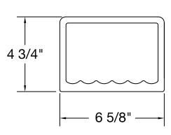
FEATURES Dimensional Tolerance ± 1/6". Dimensions needed for site preparation should be measured from the unit. American Bath Group assumes no responsibility for preparatory work.
