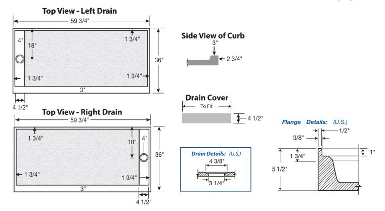
FEATURES Dimensional Tolerance ± 1/8". Dimensions needed for site preparation should be measured from the unit. American Bath Group assumes no responsibility for preparatory work.
