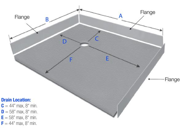
$\textbf{FEATURES} \ \ \text{Dimensional Tolerance} \ \pm \ 1/4\text{".} \ \ \text{Dimensions needed for site preparation should be measured from the unit. American Bath Group assumes no responsibility for preparatory work.}$
