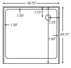
Note: Drain opening is NOT a standard drain opening. This pan can only be used with the Winglt drain listed below
