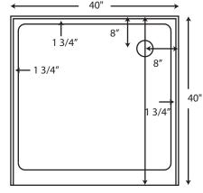
Note: Drain opening is NOT a standard drain opening. This base can only be used with the Winglts Vortex Shower Drain pictured below.
