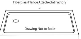
Integral 3 1/4" Curb Left Hand Drain Shown. Left & Right Hand Drain Available
