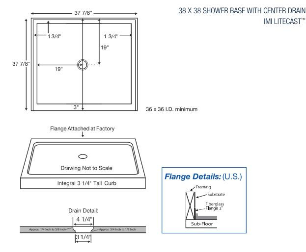
FEATURES Dimensional Tolerance ± 1/6". Dimensions needed for site preparation should be measured from the unit. American Bath Group assumes no responsibility for preparatory work.
