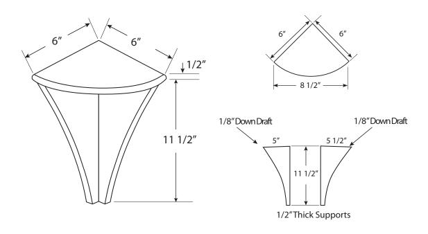
$\textbf{FEATURES} \ \ \text{Dimensional Tolerance} \ \pm 1\%". \ \ \text{Dimensions needed for site preparation should be measured from the unit. American Bath Group assumes no responsibility for preparatory work.$
