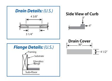
FEATURES Dimensional Tolerance ± 1/8". Dimensions needed for site preparation should be measured from the unit. American Bath Group assumes no responsibility for preparatory work.
